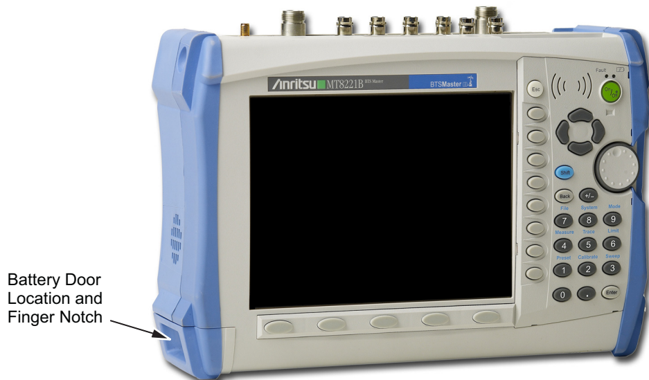
Figure 4-1. Battery Access Door Location and Finger Notch
