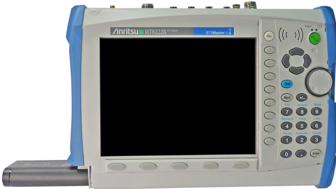
Figure 4-4. Removing the Battery
