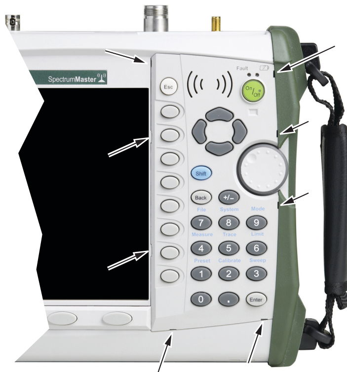
Location of the 8 tabs holding the keypad bezel
